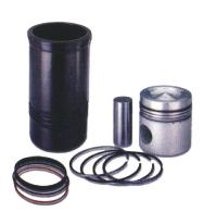
Chromium - Iron alloy and produced by centrifugal casting. The inner wall of the liner is coated with Lubrite for quick break-in and better resistance to wear and scuff.
